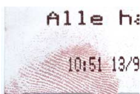
Detail of queue ticket developed with ThermaNin in petroleum ether.
