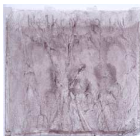
Queue ticket developed with a regular ninhydrin solution (heptane, ethanol, ethyl acetate, acetic acid)
