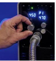
A completely new user interface is introduced in the new PL550XL. All controls are easily accessible through 3 rotary dials. The main dial is used to select the wavelength which can be used to step through the bands or rotated to jump from one band to another. Two smaller dials allow power and tuning setting to be selected. All three parameters can be read on large LED displays.
