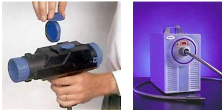
Figure 3. The excitation systems used, (left) Poliray and (right) Polilight Bluescan<sup>TM</sup>.
