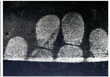
HIGHLY CONTRASTED RESULT OF THE POWDERED FINGERPRINTS ON A BLACK GELLIFTER (IMAGE REVERSED).
