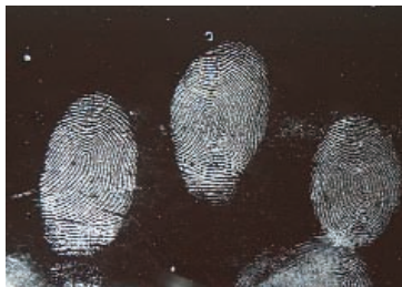
THE SAME PRINTS LIFTED AND PERFECTLY CONTRASTED ON A BLACK GELLIFTER (IMAGE REVERSED).
