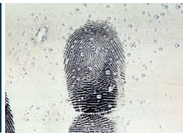
FINGERPRINTS DEVELOPED WITH MAGNETIC FINGERPRINT POWDER AND LIFTED WITH A COMMONLY USED LIFTING TAPE.
