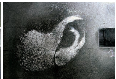
THE EARPRINT AFTER BEING LIFTED WITH A BLACK GELLIFTER (IMAGE REVERSED).
