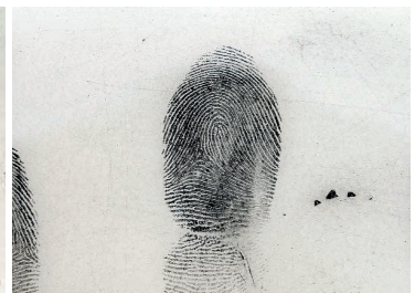
FINGERPRINTS DEVELOPED WITH MAGNETIC POWDER AND LIFTED WITH A TRANSPARENT GELLIFTER. NOTE THE ABSENCE OF AIR BUBBLES.
