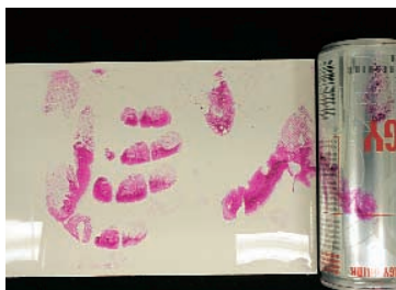
FINGERPRINTS ON SODA CAN, TREATED WITH HUNGARIAN RED AND COVERED WITH WHITE GELLIFTER; FINGERPRINTS ARE COPIED ON THE WHITE GELLIFTER.
