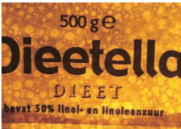
THE FINGERPRINTS STAINED. THE SURFACE HAS ABSORBED THE STAINING SOLUTION, RESULTING IN A COMPLETE LOSS OF CONTRAST.
