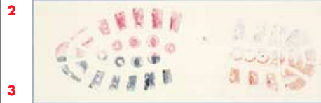
TRACES IN BLOOD, STAINED AND THEN LIFTED WITH A WHITE GELATIN LIFTER
