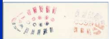
White gelatin lifters can be used for the lifting of finger- and shoeprints in blood, which are stained with protein dyes like Hungarian Red, Amido black, Crowle's stain or Coomassie blue.
