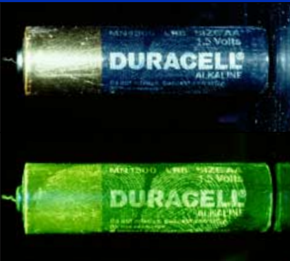
After staining the cyanoacrylate with Basic Yellow 40, more details can be seen using light of about 450 nm and a yellow filter placed in front of the camera lens.
