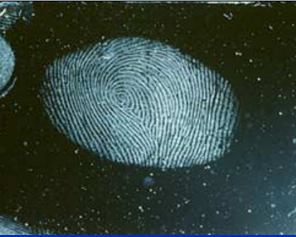
Greasy prints can be lifted even without using powder due to the extreme over-exposure that can be used in photography of traces on black gelatin lifters. Above, an example of a greasy print, lifted from glass.
