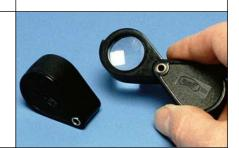
K - 1100 Coding disc with one line (Henry disc) for fingerprint magnifier K-1700.
