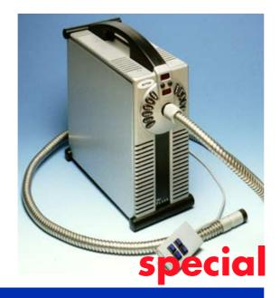
The Polilight 500 is a high-intensity light source based on a 500-watt xenon arc lamp. This type of lamp delivers UV, visible, and infrared light. A special characteristic of the light output in the visible region is that the intensity of light is the same in the whole spectrum, just like sun light. This is in contrast with halogen lamps that deliver progressively more light, going from blue (low wavelength) to red (high wavelength).
