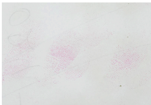
Fingerprints on white paper developed with 1,2-IND (IND-Zn formulation)
