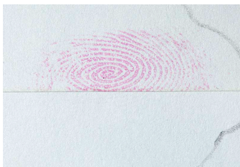
Fingerprint cut in half and treated with DFO (bottom) and 1,2-IND (top - IND-Zn formulation)
